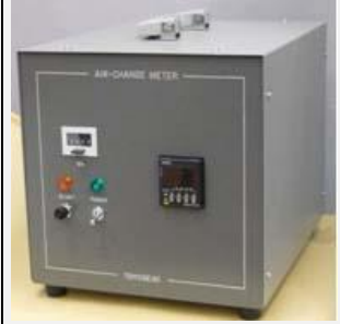
7, 8. Portable air change meter
